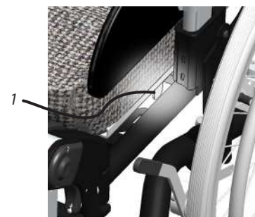
Diagram 20. The lever (1) for seat depth adjustment is located under the left side of the seat.
